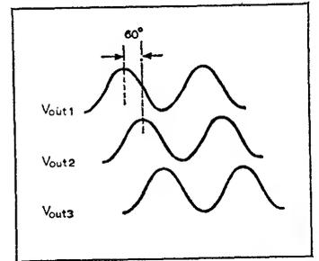
and maintaining as close a ratio as possible between the R values. Frequency is approximately  $1/3RC$ . Note that with the CR values necessary for  $60^\circ$  phase shift at a specific frequency, the output of each buffer stage is attenuated by about one half and hence the minimum gain of each stage must be  $> 2$ .
