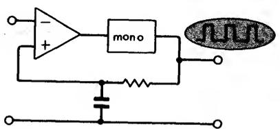
Fig. 9. Monostable circuit produces output pulse when input exceeds a certain level, in either sense.
