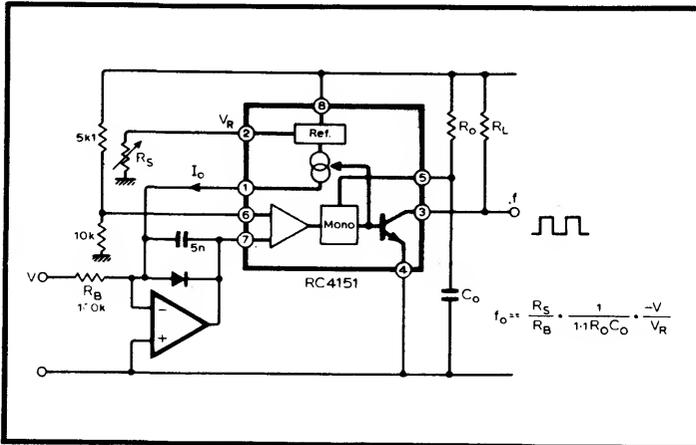
The new generation of linear integrated circuits includes complete v-f modules that will compete with the hybrid and modular versions for many applications. One such monolithic device RC4151 is in line of succession to the 555. It includes a monostable comparator and output stage, but adds a switched current generator. It can be used without additional active devices, but for improved linearity is combined with an op-amp to form a charge-balancing system. The input
