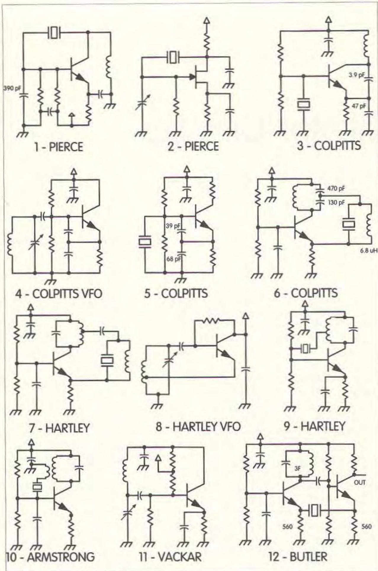
Fig. 1. Common—and not so common—transistorized oscillator circuits.
