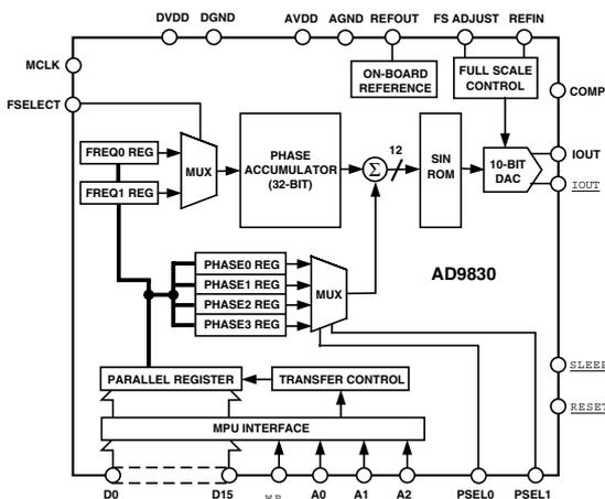
Figure 2. Block diagram of AD9830 50-MHz C-DDS.
