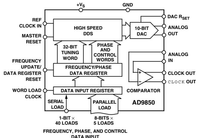
Figure 3. Block diagram of AD9850 125 MHz C-DDS.
