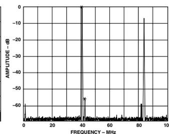
Figure 5. AD9850 wideband spectral plot at 40 MHz Aout (125-MHz clock).
