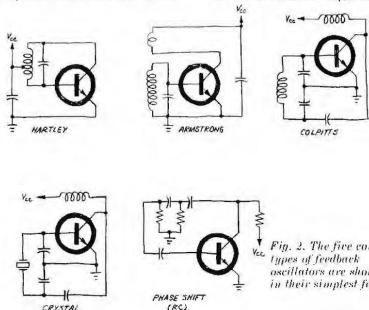
Fig. 2. The five common types of feedback oscillators are shown in their simplest forms.
