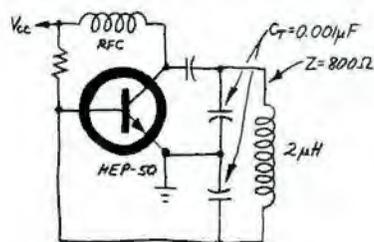
Fig. 3. Start with this basic Colpitts oscillator circuit.
