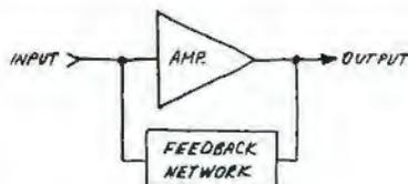
*Fig. 1. Basic oscillator is amplifier with feedback.*
