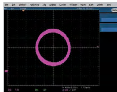
Figure 3 When swept in frequency, the phase varies from -89 to -91^\circ .
