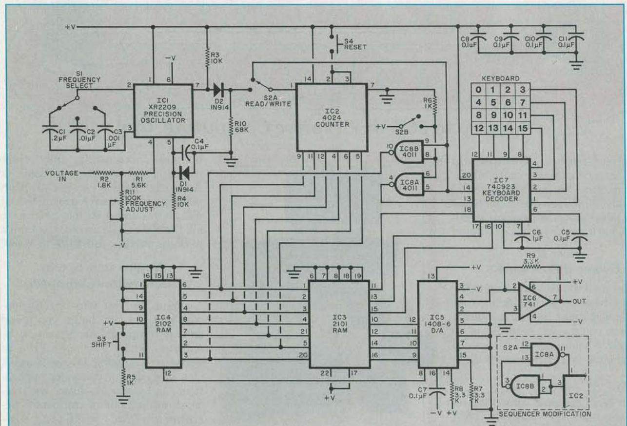
Fig. 2. The vco produces a square-wave output whose frequency is proportional to the input voltage.
