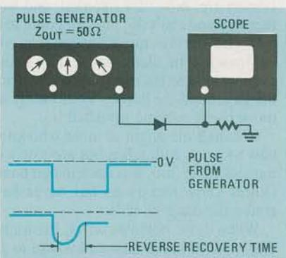
**FIG. 14—MEASURING DIODE reverse-recovery time.** A 100-nanosecond pulse-width with a duty cycle of less than 1 percent should be used. The generator rise time should be less than the expected reverse-recovery time. The positive pulse offset is set to generate the specified forward current. A 60-ohm resistor converts the output current to voltage for display on the oscilloscope.
