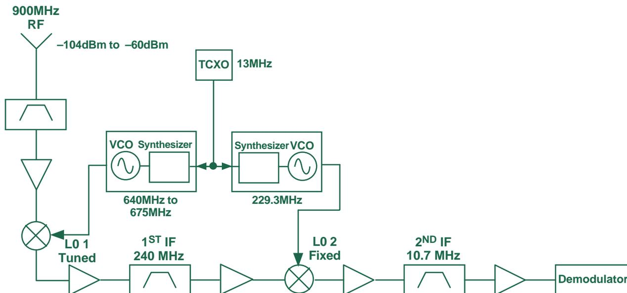
Figure 4. Signal chain for GSM base-station receiver.
