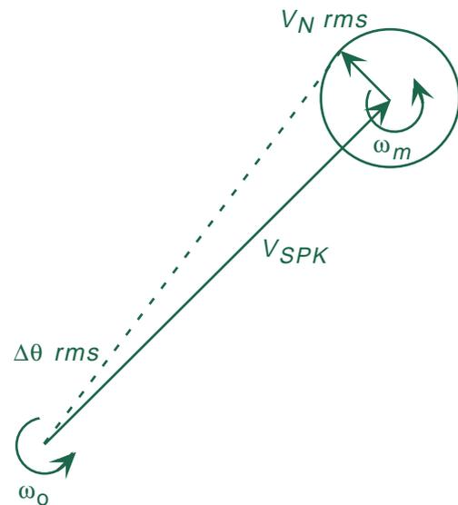
Figure 2. Phasor representation of phase noise.
