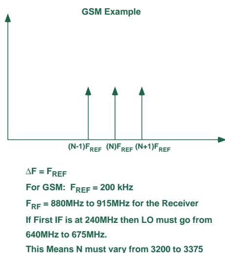
Figure 5. Testing frequencies for GSM base-station receiver.
