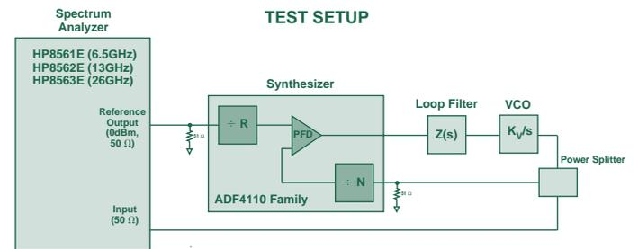
Figure 7. Measuring phase noise with a spectrum analyzer.
