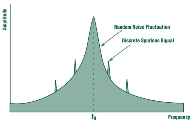
Figure 1. Short-term stability in oscillators.
