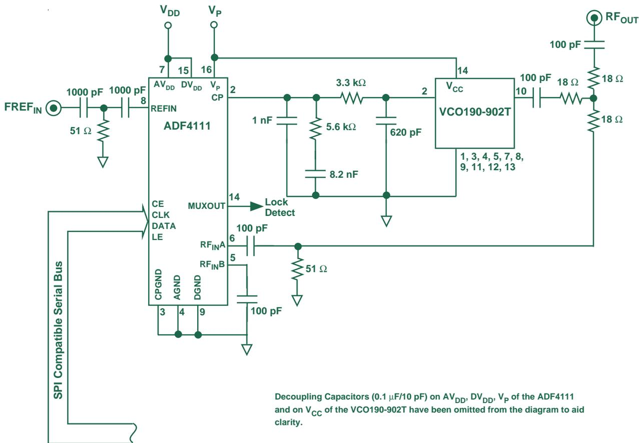
Figure 6. Transmitter local oscillator for GSM handset.
