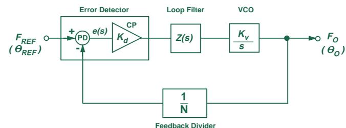
Figure 2. Basic phase-locked-loop model.
