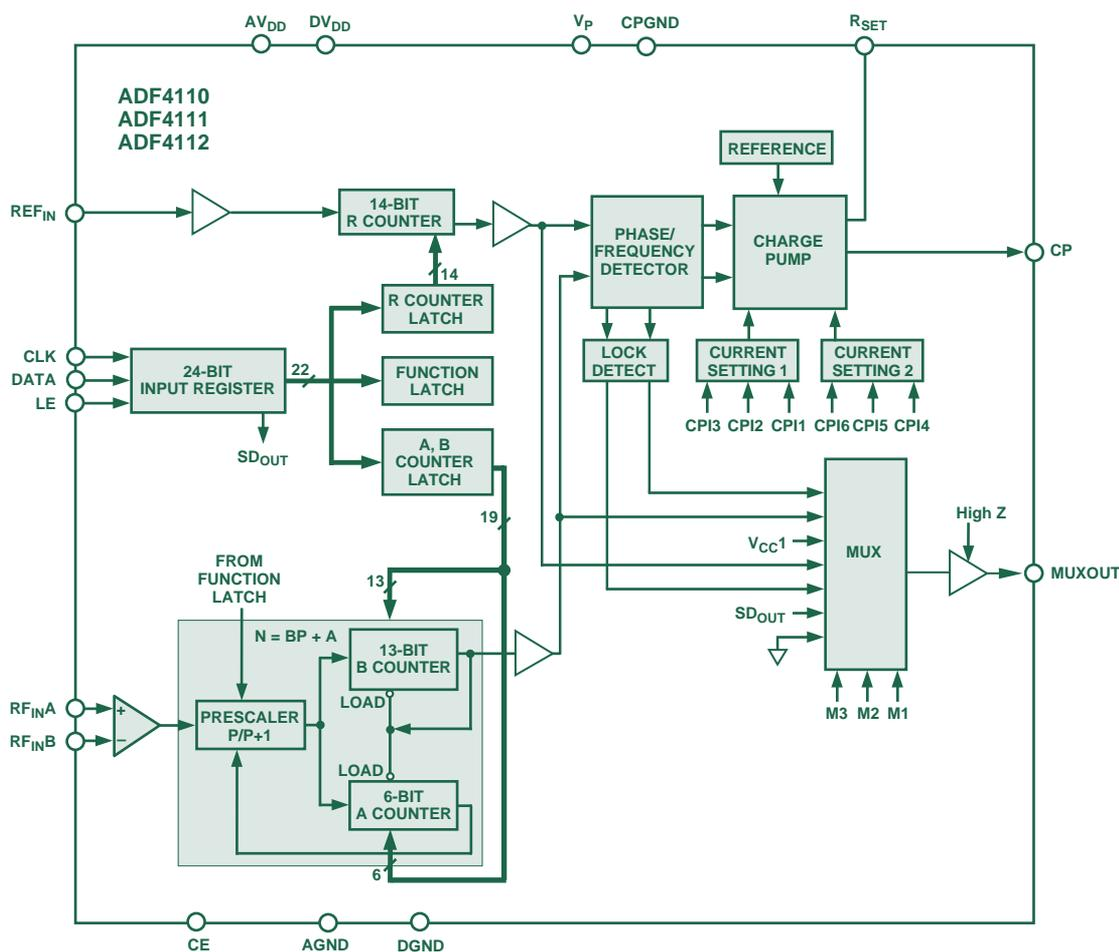
Figure 7. Block diagram for the ADF4110 family.
