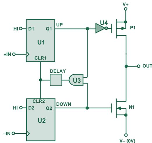
Figure 1. Typical PFD using D-type flip flops.
