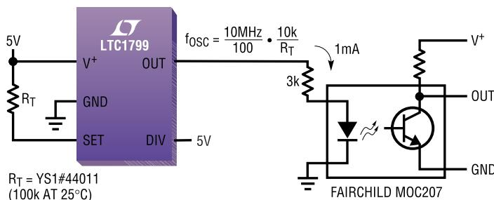
Figure 7. Remote Thermal Sensor Using a Thermistor
