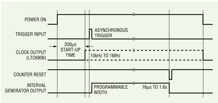
Figure 4. Timing Diagram for Time Interval Generator
