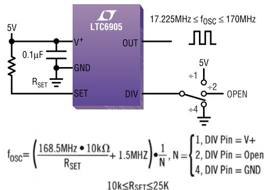
Figure 2. Resistor Set Oscillators
