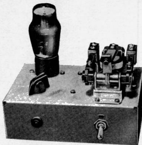
The light-sensitive unit—photocell is held in place by rubber grommet.
