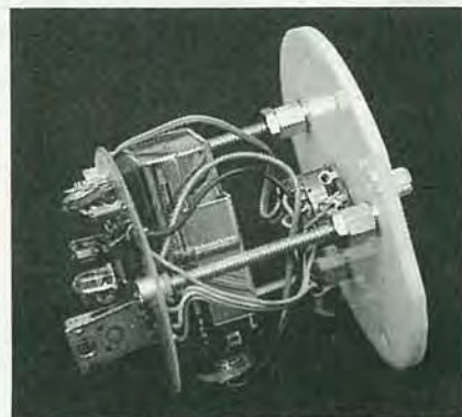
FIG. 4—THE TRANSMITTER ASSEMBLY. It is fitted inside one end of a rugged cardboard tube that has a collimating lens at the other end.
