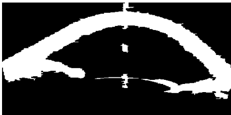
Fig. 3-26 A binary image originated from the original image after the binarisation with a threshold of 90% of the maximum value
