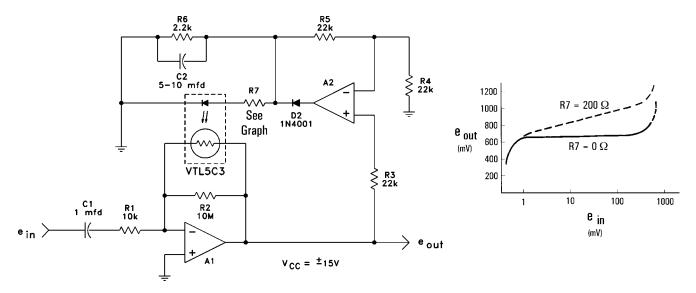
Figure 4a. Peak Sensing Compressor
