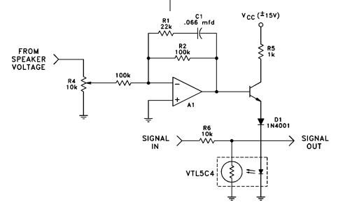
Figure 8a. Speaker Power Limiter with Frequency Compensation
