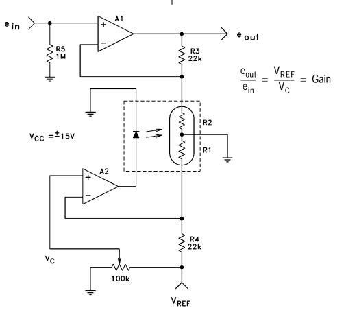
Figure 10. Electrically Programmable Gain
