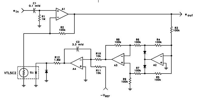
Figure 9. AGC Circuit with Electrical Setpoint
