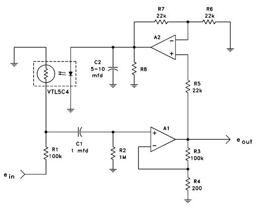
Figure 5. Peak Sensing Compressor with Constant Bandwidth
