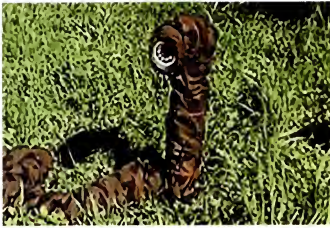
Snake Robot in its natural habitat. Note how the robot has its body raised to get a better view with the head mounted camera.
