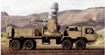
Centurion C-RAM is a land-based version of Phalanx, used for automated base defence against artillery.
