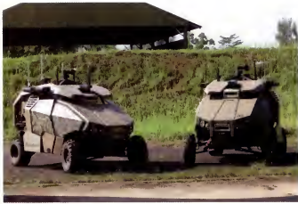
The G-NIUS Guardium is a fully autonomous vehicle which can patrol a route, detect and fight off intruders.
