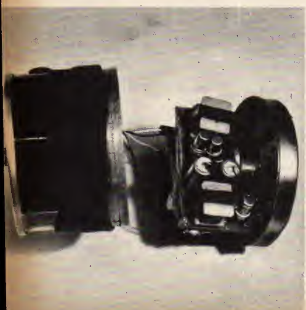
Fig. 6. This illustrates the technique used in detecting hidden radio microbugs. The hidden snooping device is activated by the operator whistling in a "suspect" area. This sound is transmitted by the bug, and received by the locator, the audio output of which is picked up by the bug, and so a self-sustaining feedback loop is created around the two devices. The intensity of the loudspeaker output will increase as the locator is brought closer to the concealed bug, whose hiding place is thus soon discovered
