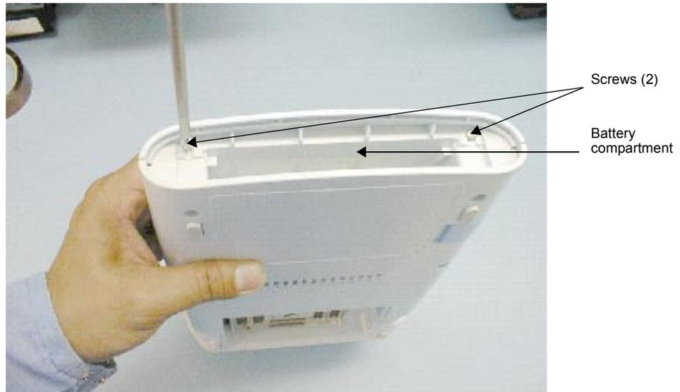
**Figure 7.17** Replacing the Control Panel
