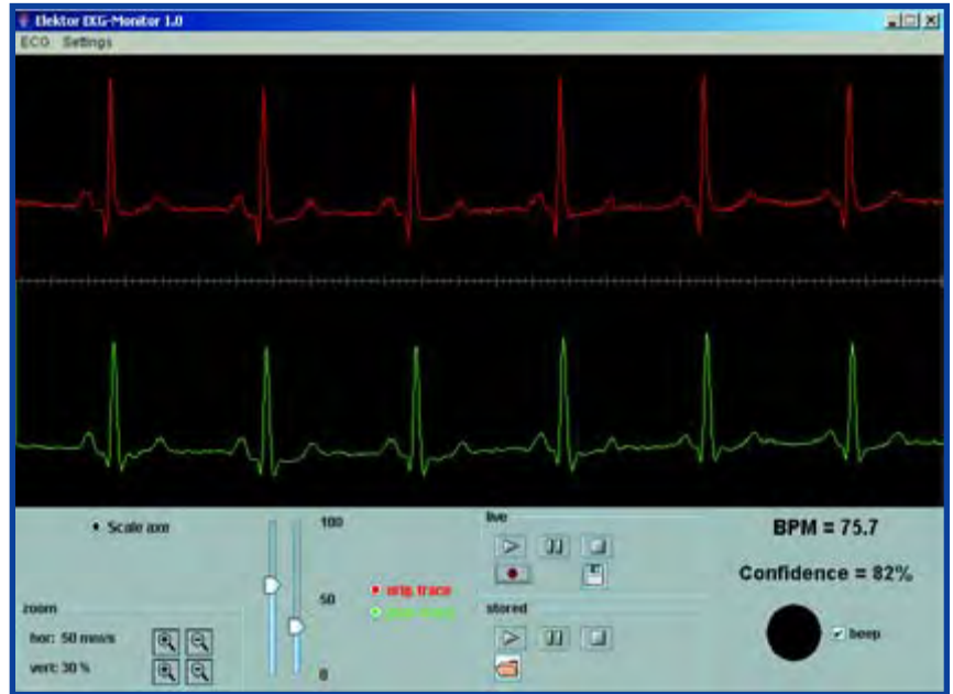
Figure 7. The main program window shows the original signal (above) and the processed signal (below).
