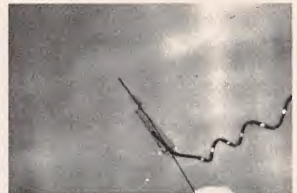
The neurotrophic electrode shown here is the key development in a new system that could someday help paralyzed individuals communicate with the world around them.
