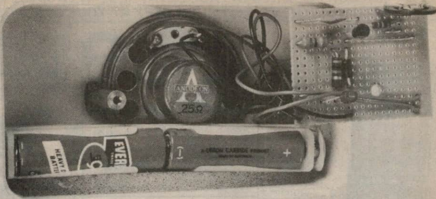
A view of our mosquito repeller, taken with the back off and the board swung out. Almost any small speaker can be used, as the text explains.
