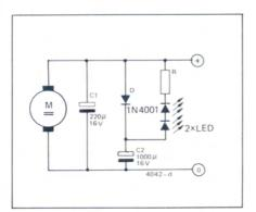
across M and  $C_2$  discharges via the two LED's, resistor R, and motor M. If braking is the result of a short-circuit of the supply voltage, both capacitors discharge via the short-circuit connection; in that case the LED's burn somewhat brighter. The value of resistor R can be calculated with the following simple formula:
