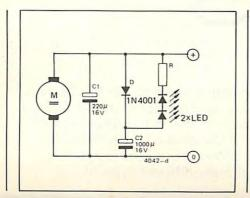
across M and C2 discharges via the two LED's, resistor R, and motor M. If braking is the result of a short-circuit of the supply voltage, both capacitors discharge via the short-circuit connection; in that case the LED's burn somewhat brighter. The value of resistor R can be calculated with the following simple formula:
