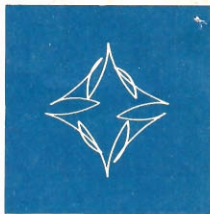
Fig. 6. Diamond-shaped pattern results when offset controls are at opposite settings.
