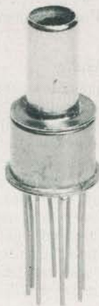
FIG. 2—THE LX0503A pressure transducer is ideal for barometric applications.
