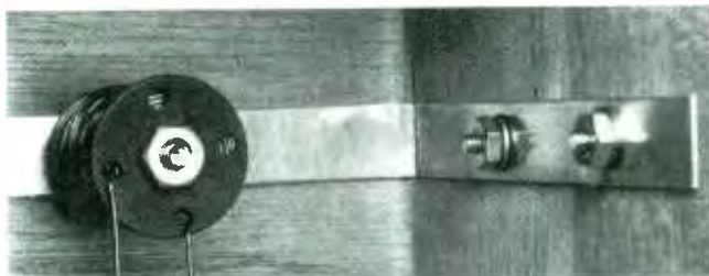
When the coil bracket is secured inside the cabinet, you should make sure the coil is right up against the top of the cabinet. A good, snug fit along the sides is also desirable.
