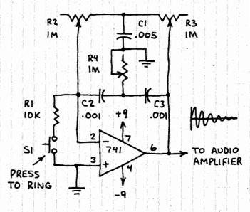
ADJUST R3 TO JUST BELOW OSCILLATION POINT. ADJUST R2 AND R3 FOR SOUNDS SUCH AS BELL, DRUM, TINKLING, ETC.
