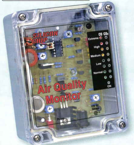
Below: the completed prototype with the label in position. The "light pipes" fitted to the LEDs ensure that only the correct "dots" on the bargraphs are lit.
