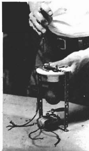
Bracket shaped from pipe-hanger iron supports the motor and lamp. Wrap part of the top of the bracket with tape to prevent shorts.
