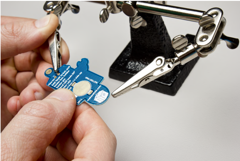
Figure 2-2. Holding a PCB in the helping hands
