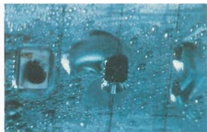
Figure 1. Surface tension can cause flux volatiles to bubble around SMT components, resulting in solder skips and bridges.
