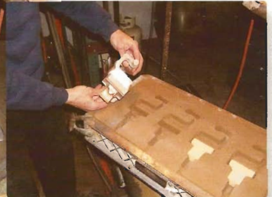
The sand casting shows how the cores are placed in the production mold. The technician is holding a completed casting.
