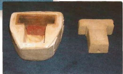
The core print sits next to the core box it was made from.
