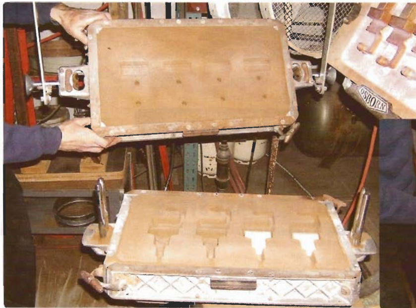
This shows the green sand-production mold after removal of the pattern, before closing.
