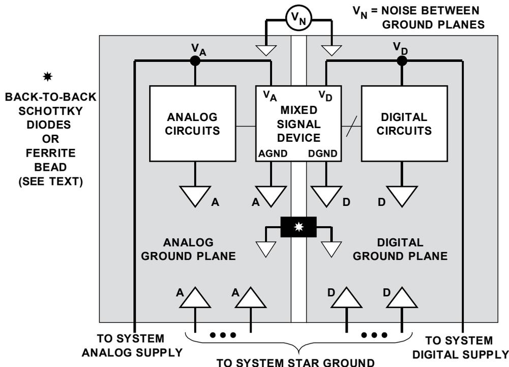
Figure 12.58: High Digital Currents: Multiple PC Boards
