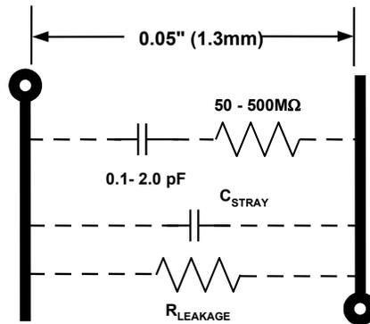
**Figure 12.17:** *DA Plagues Dynamic Response of PCB-Based Circuits*
