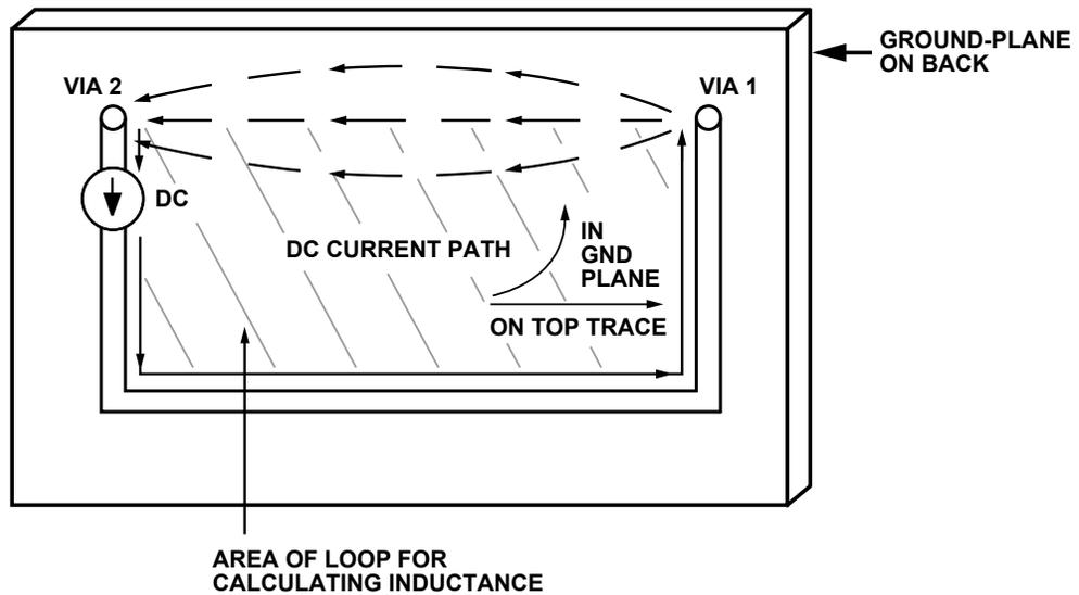
**Figure 12.61:** DC Current Flow for Figure 12.60
