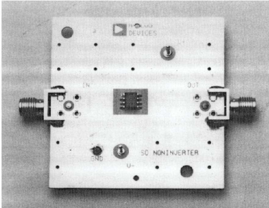
**Fig. 12.30a:** AD8001AR (SOIC) Evaluation Board—Top View
