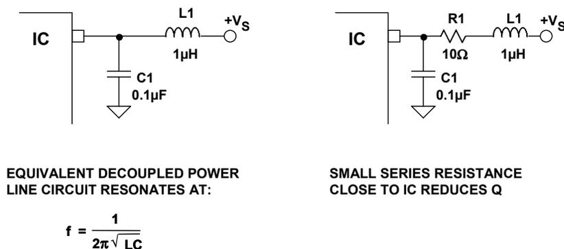
**Figure 12.69:** Resonant Circuit Formed by Power Line Decoupling
