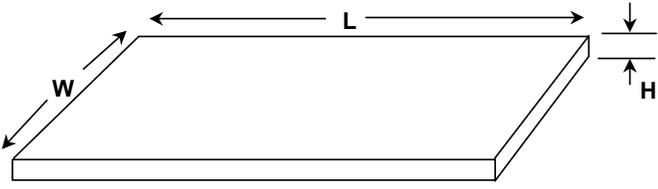
$$\text{STRIP INDUCTANCE} = 0.0002L \left[ \ln \left( \frac{2L}{W+H} \right) + 0.2235 \left( \frac{W+H}{L} \right) + 0.5 \right] \mu\text{H}$$
