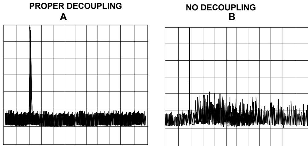
VERTICAL SCALES: 10dB/div, HORIZONTAL SCALES: 10MHz/div
