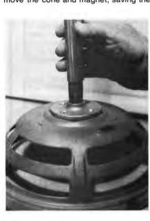
latter for use in your shop to mount tools on a wall, keep machine hardware in one place, etc. Now, substitute a ½" (12.7-mm) diameter pipe fitting for the magnet, using a threaded flange, as shown in the photo. Fasten the speaker basket to the roof with pan-head sheetmetal screws. Assemble the antenna, fasten it to the mast, and slip the mast over the pipe fitting. Aim the antenna in the desired direction and clamp and guy the mast.—Glen Stillwell, Manhattan
