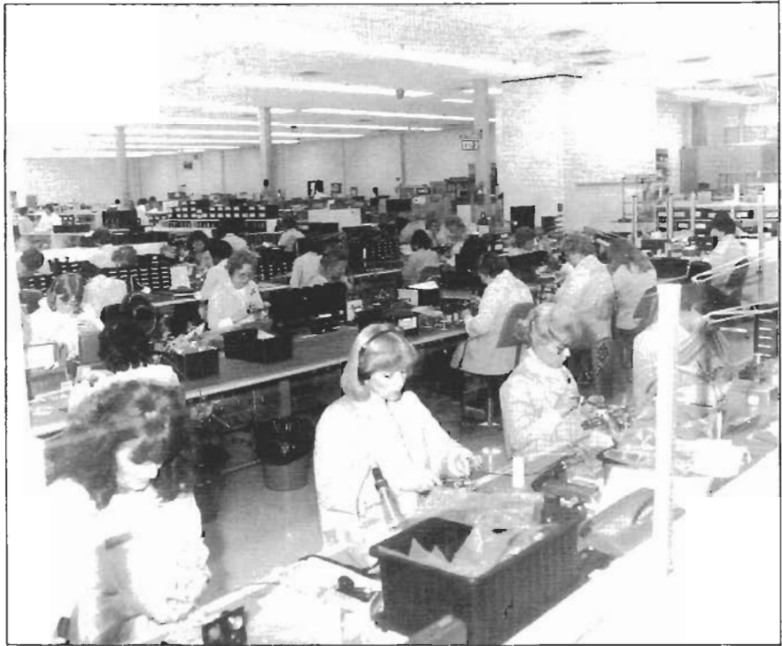
Static protective boxes are much in evidence here
