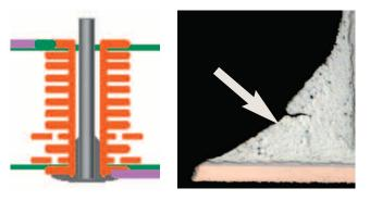
Figure 4: Examples of insufficient hole fill and fillet cracking
