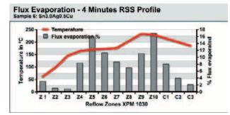
Figure 2. Ramp Soak Spike Profile
