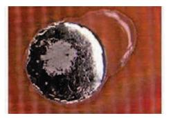
Figure 1. Lead Free Solder Joint with Flux Residue
