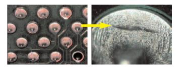
Solder shrinkage effects on solder joints.
