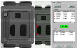
Figure 18 Poorly formed source joint - 11% missing
