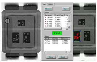
Figure 13 Voids on the left source contact
