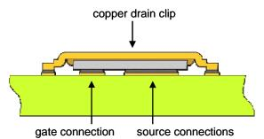
Figure 1 Side view of DirectFET device
