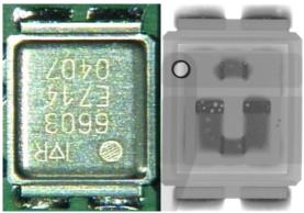
Figure 8 Rotated device Reject all rotated devices.
