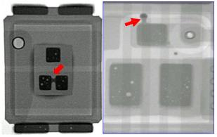
Figure 21 Examples of short circuits
