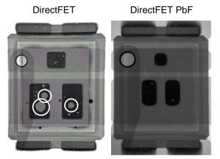
Figure 11 Examples of solder voids
