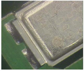
Figure 3 External solder fillets on the drain
