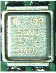
Figure 4 Self-centered with good solder fillets
