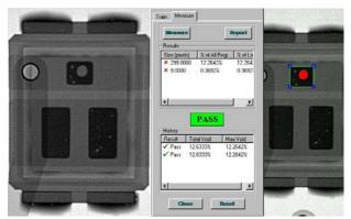
Figure 12 Voids on the gate contact
