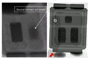
Figure 20 Examples of open circuits
