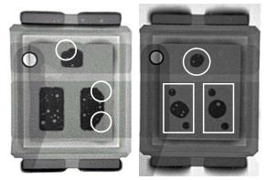
Figure 16 Examples of poorly formed joints
