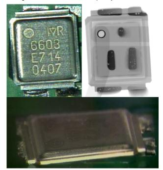
Figure 10 Twisted and tilted device
