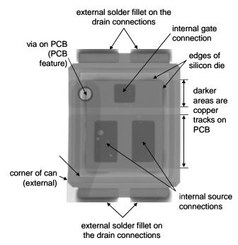
Figure 6 Features revealed by an X-ray
