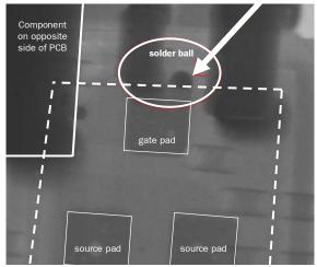
Figure 15 Example of a problematic solder ball
