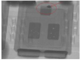
Figure 22 Over-sized gate pad on PCB
