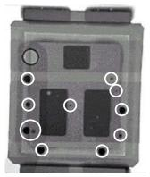
Figure 14 Examples of solder balls
