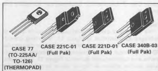
Figure 13. Plastic Body-Mount Packages
