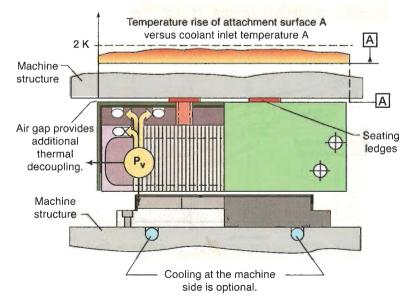
Coolant should only be a few degrees cooler than ambient temperature, to avoid condensation.
