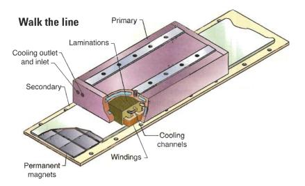
The overall height, tube diameter, and length of the cooling system determines the pressure drop of coolant — and appropriate pump size.
