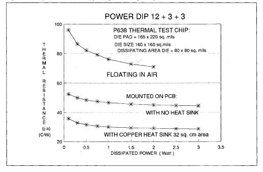
Figure 6 - Rth(j-a) of DIP (12+3+3) package vs. dissipated power
