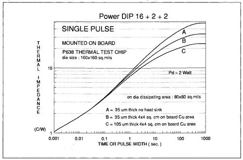
Figure 10 - DIP 16+2+2 Transient thermal resistance for single pulses
