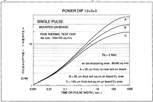
Figure 11 - DIP 12+3+3 Transient thermal resistance for single pulses
