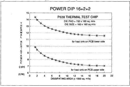
Figure 3 - POWER DIP 16+2+2 Rth(j-p) vs on die dissipating area
