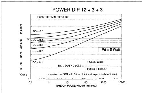
Figure 14 - Peak transient thermal resistance of DIP (12+3+3)
