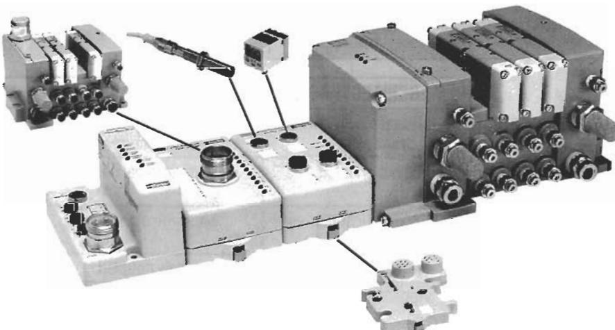
Parker's Isysnet Field Bus System includes a valve drive module that controls up to 32 solenoids; I/O modules with up to 256 inputs and 256 outputs; and communications modules using EtherNet/IP, ControlNet, DeviceNet, and Profibus DP. The plug-in pneumatic valves meet ISO 15407 and 5599 dimensional and electrical standards.
