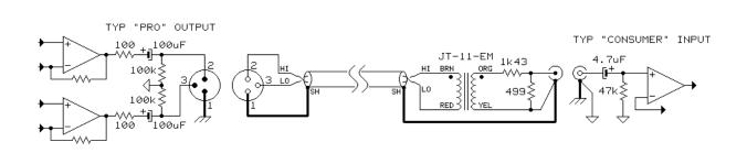
3.1 - "BETTER" uses an Output Transformer and a "Pad"
