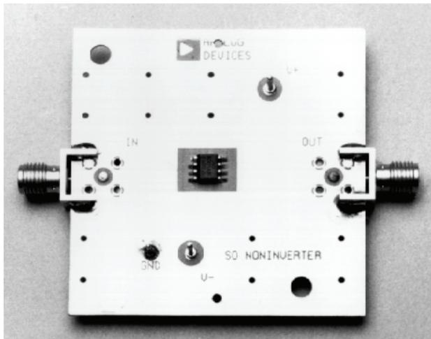
**Figure 13.52:** *The AD8001 Evaluation Board Top View*
