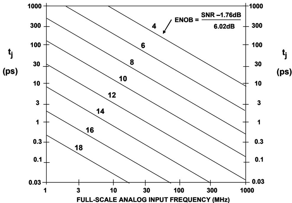
**Figure 13.18: SNR vs. Input Frequency vs. Jitter**
