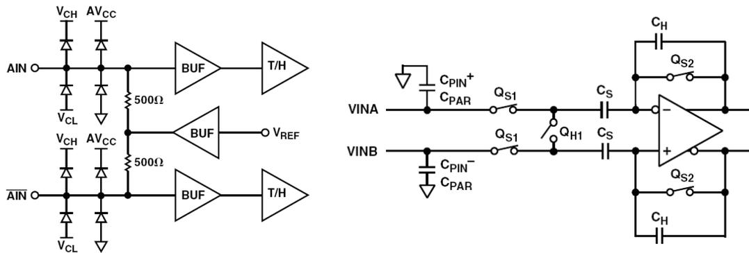
*Note: Different input data structures showing those that are both connected to the internal common-mode voltage (on the left) and those that are not (on the right).*
