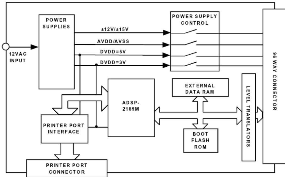
**Figure 13.59:** Precision ADC Controller/Evaluation Board
