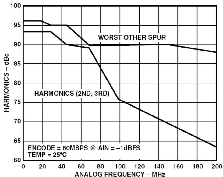
**Figure 13.16: Example Converter Performance vs. Analog Input Frequency**
