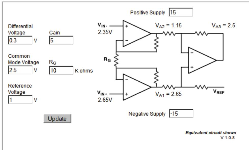
Figure 13.33: Instrumentation Amplifier Common-Mode Range/Gain/Noise Calculator Screen
