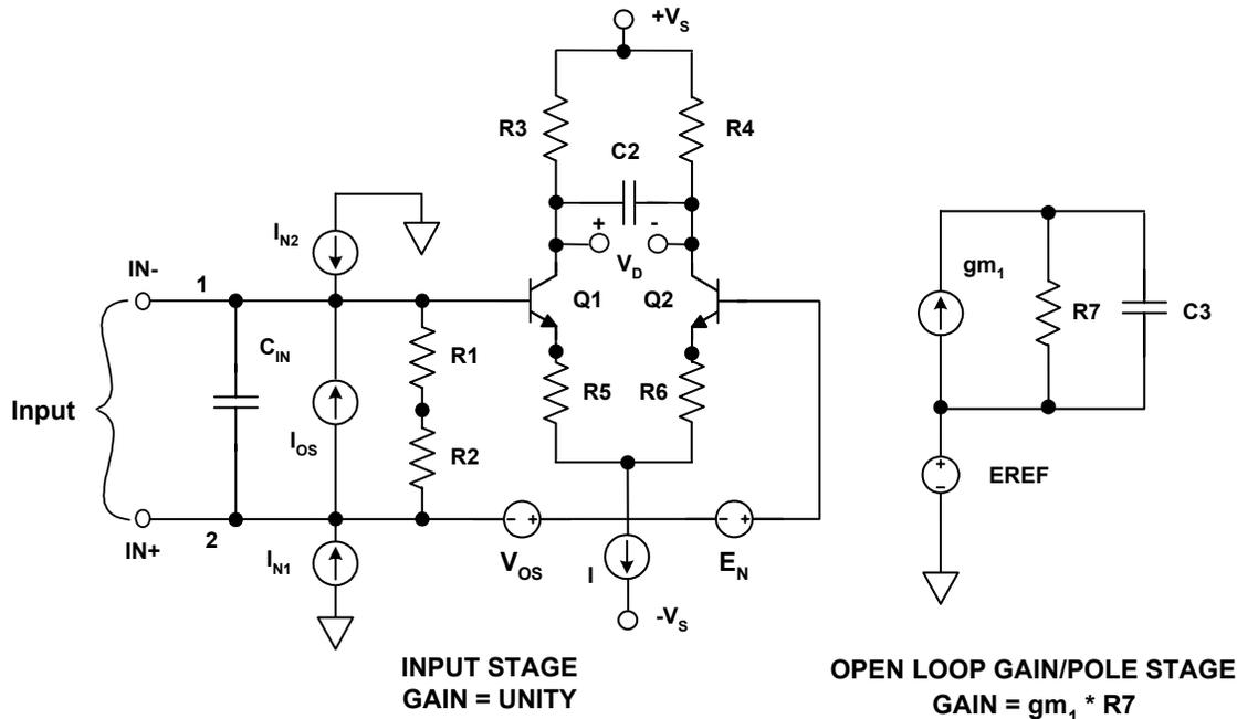
**Figure 13.2:** Input and Gain/Pole Stages of ADSpice Macromodel
