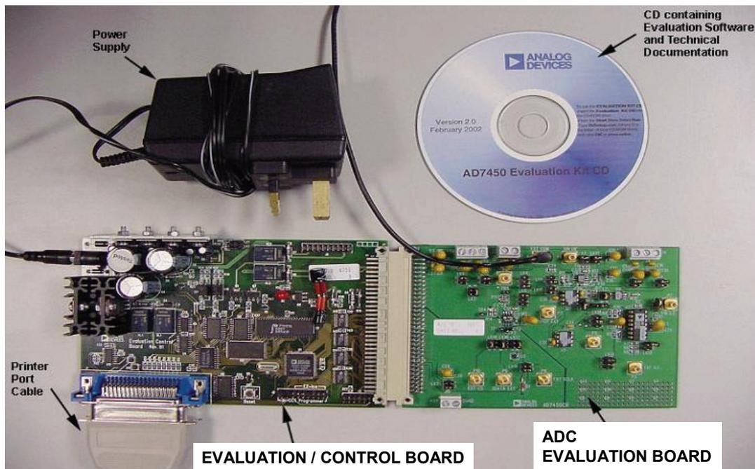
**Figure 13.55:** Evaluation/Control Board and ADC Evaluation Board for ADCs
