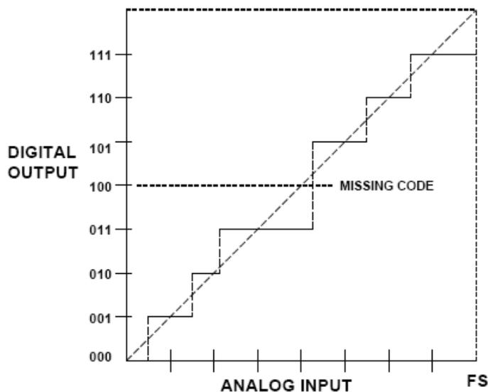
Figure 13.17: Data Converter Transfer Function
