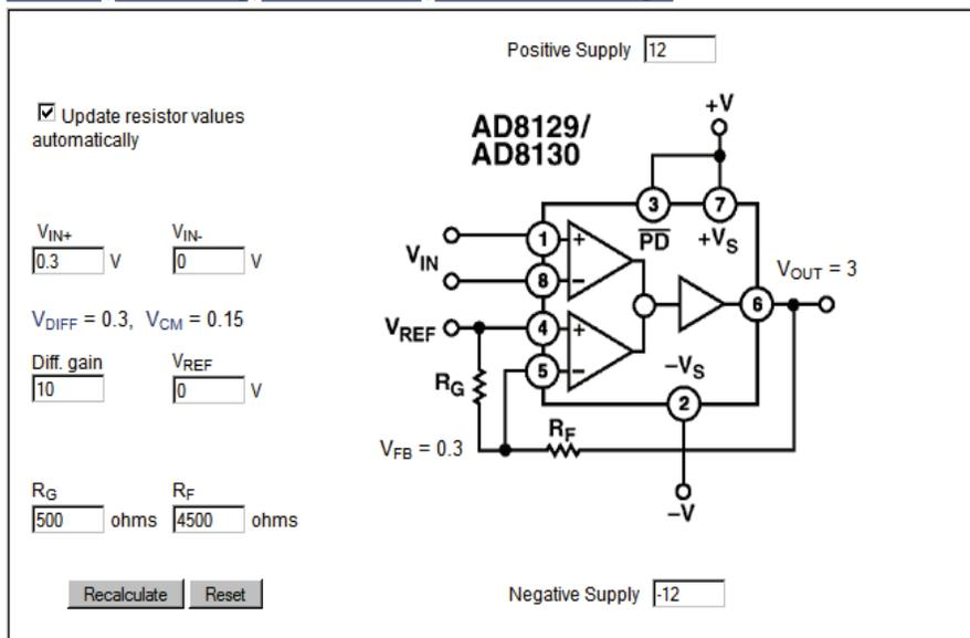
Figure 13.35: Active Feedback Common-Mode Range/Gain Calculator Screen
