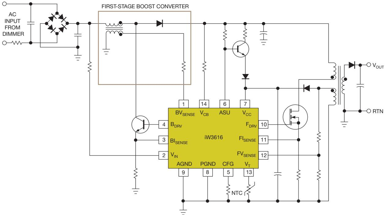
**Figure 3** The circuit in this example of a two-stage, high-power-factor-correction LED driver (the iW3616) uses an NTC resistor to provide LED overtemperature protection and derating, thus extending bulb lifetime.
