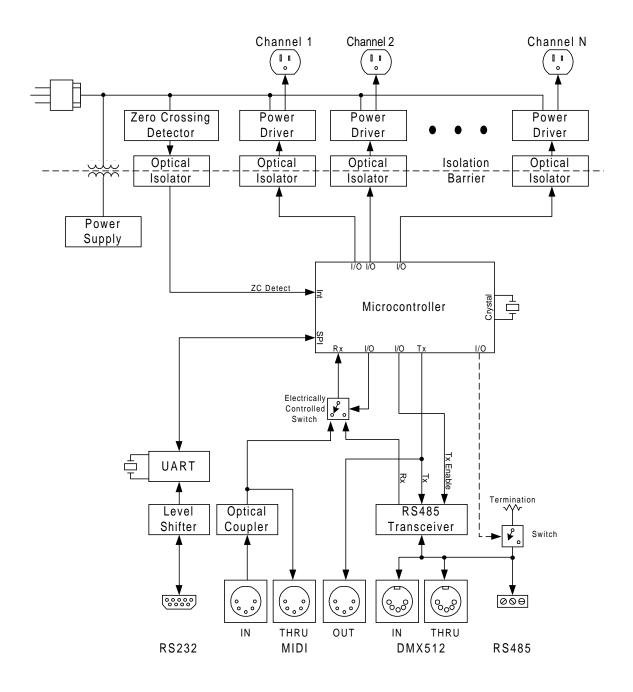
Figure 3: Dimmer block diagram
