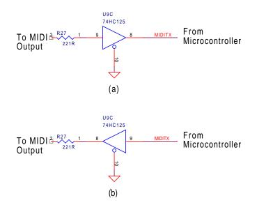
Figure 17: Logic gate U9C - (a) incorrect (b) correct
