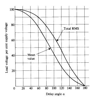
Figure 2: Load Voltage vs. Delay Angle
