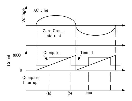
**Figure 5: Phase Control Comparator Operation**
