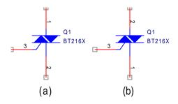
Figure 15: Triac pinout - (a) incorrect (b) correct
