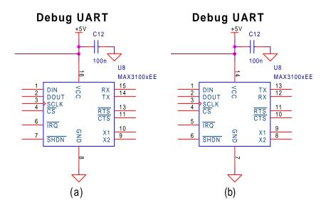
Figure 14: Debug UART pinout - (a) correct (b) incorrect
