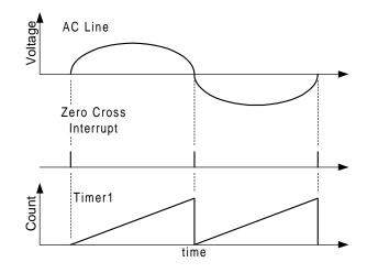
Figure 4: Phase Angle usage of Timer/Counter1
