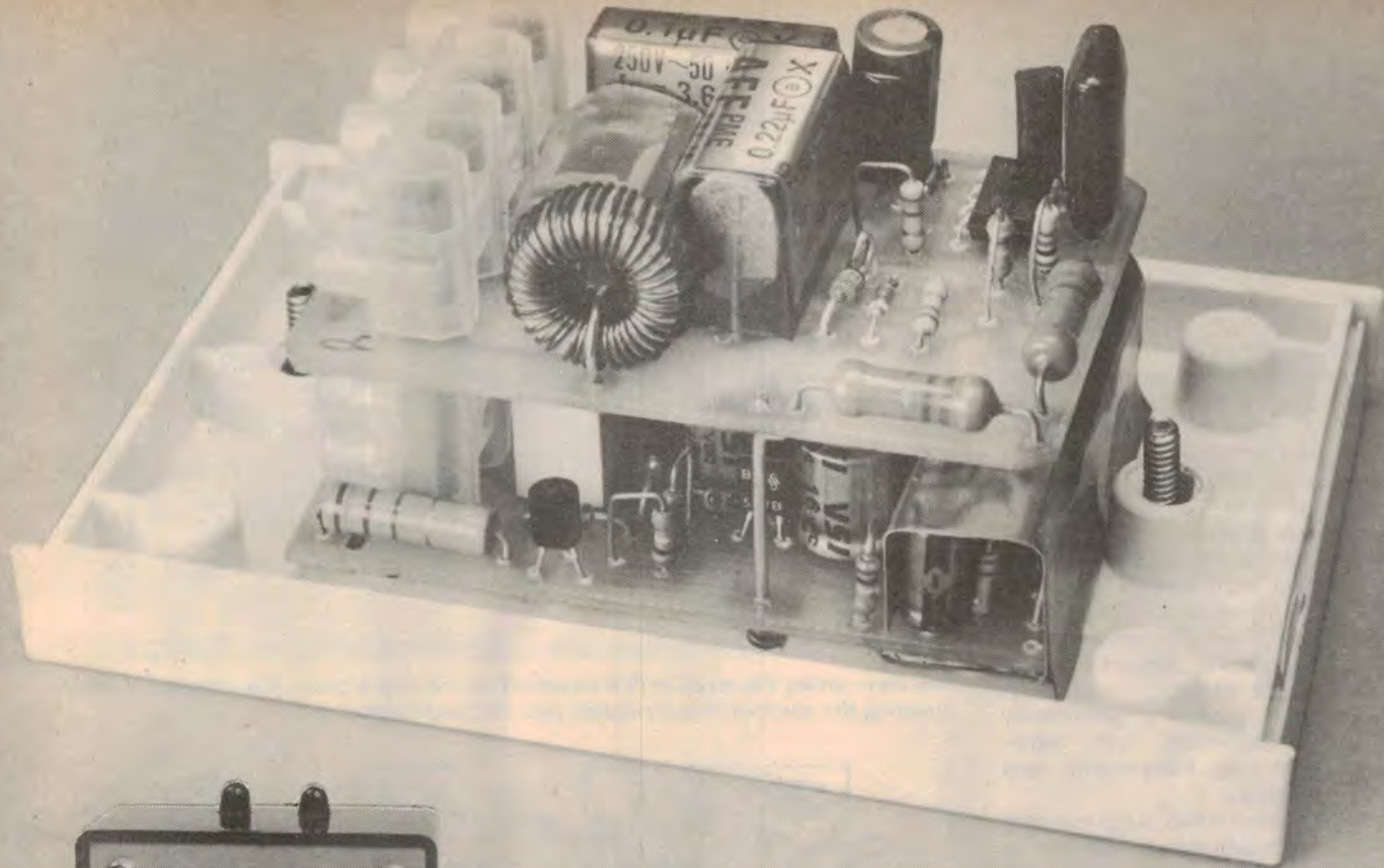
The remote control receiver PCB and the dimmer PCB are both mounted on the back of the switch plate. At left is the hand-held infrared transmitter.
