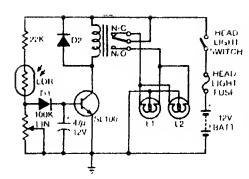
The circuit also operates without the power transistor 2N3055 (a saving). The LDR can be mounted on a small bracket screwed to the right head lamp's mounting screw after wrapping the t.DR neatly in a single layer of polythene sheet.
