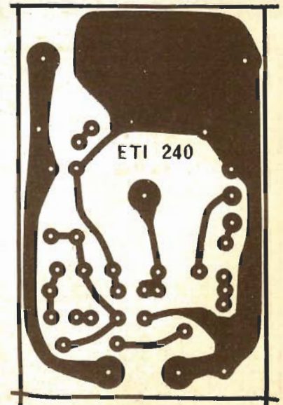
Fig. 4. Printed-circuit layout for the flash. Full size 73 x 47 mm.
