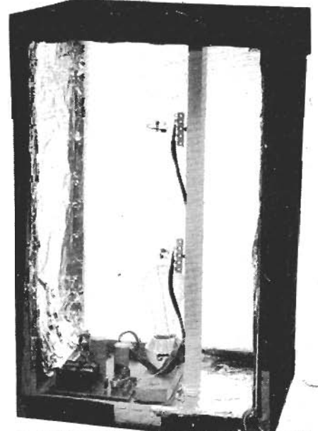
The interior of the softbox, showing the perf-board, 150W lamp and two 50W/S tubes.
