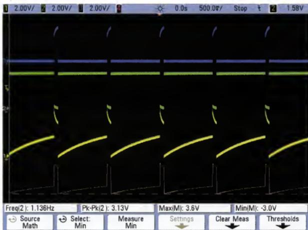
Fig.3: scope grab showing the critical voltages. The blue trace is pin 7 (GP0), green trace is pin 2 (GP5), yellow trace is the positive terminal of capacitor C1 while the mauve trace is the voltage across LED1 and R2. This shows a peak value of 3.6V, despite the 3V supply.
