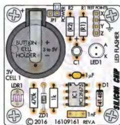
Fig.4 (left): the larger of the two flasher boards. Use this as a guide during assembly and take care with the polarity of IC1, C1, D1 and ZD1.
