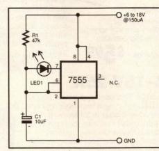
whilst consuming only 150uA from the supply. The circuit can be pow ered from 6 to 18 volts, and while pin 3 is not used here, there is no reason why its output could not be used fo other purposes.
