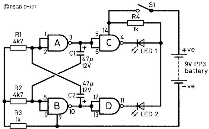
**Figure 1** Flashing LEDs, circuit diagram
